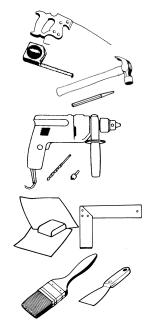
**Tape measure** Cordless drill / driver and bits Hand saw or power mitre saw **Claw hammer** Nail punch Sanding block 4cm dowel Sandpaper (80, 120, 280, 400 grades) **Try-square** Putty knife 75mm paint brush
