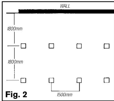
Once the plate has been fixed and bearer height has been determined, transfer this onto other stumps using a straight edge and level or string line and level. Mark with a square and cut off stumps to correct height.
